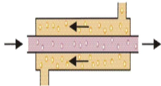
Figure 1 Countercurrent flow
