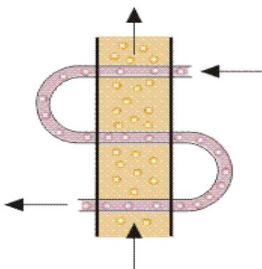
**Figure 4 Cross Counter flow**
