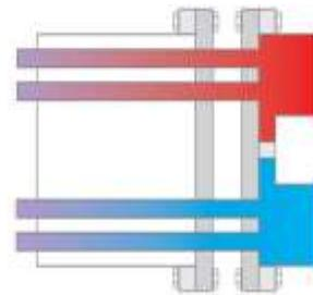
**Figure 9 Single tube sheet Design**
