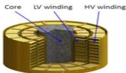
**Figure 1** Disc winding transformer
