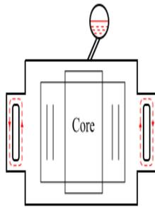
**Figure 2 Transformer cooling by a natural oil circulation system**
