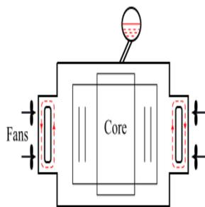
**Figure 3 Transformer cooling by natural oil circulation and strike of air.**
