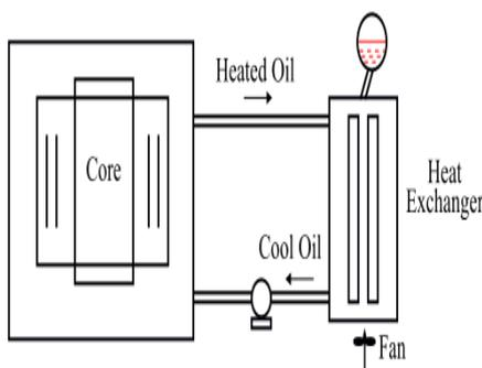
**Figure 4 Oil Forced Air Forced Cooling**
