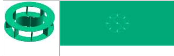
Fig. 4: CAD model of two blades with wind booster for VAWT
