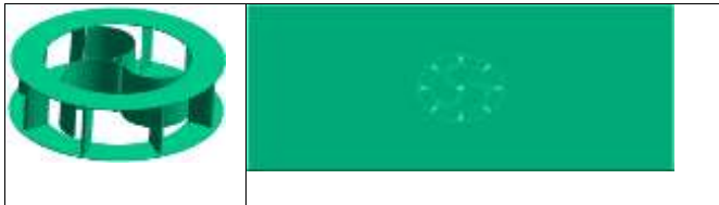
Fig. 8: CAD model of three blades through wind booster for VAWT
