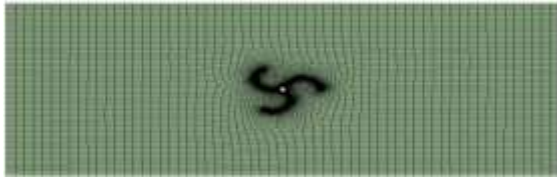
Fig. 7: Meshing of two blades lacking wind booster for VAWT
