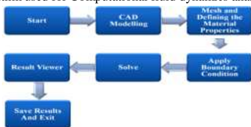
Fig. 1: Algorithm employed for Computational fluid dynamics analysis
