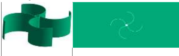
Fig. 10: CAD model of four blades without wind booster for VAWT
