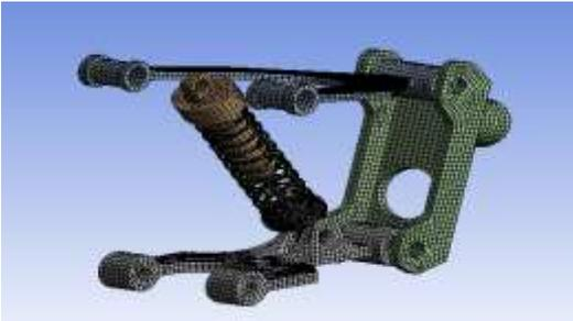
Fig. 8 Meshing: Over-all No. of Nodes: 61915 & Over-all No. components: 160624
