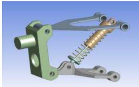
Fig. 5 Only one spring model arranged in Catia
