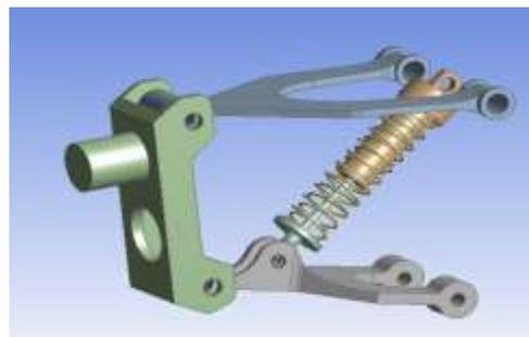
Fig. 6 Dual spring model arranged in Catia
