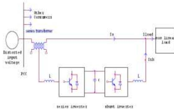
Fig. 1 proposed PQ compensation with load circuit diagram
