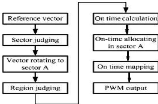
Fig. 3 SVPWM Simplified for the three level calculation flow
