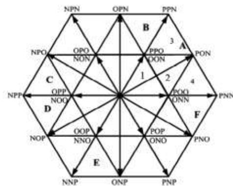
Fig. 2 Space-vector diagram of the three-level converter
