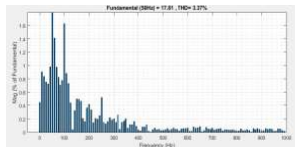
Fig. 25 THD% measured of current in system with (DMS-PSO) control for quality enhancement
