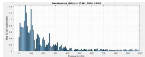
Fig.33 THD% in current in the system with (NMS-PSO) control for quality enhancement
