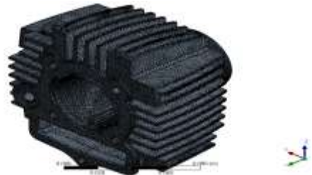
Fig. 17: Meshing of proposed design -2 with water jacket The total node is generated 972853 and the total number of elements is 560322.
