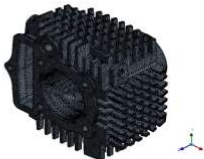
Fig. 23: Meshing of proposed design-3 of engine block The total node is generated with 938346 and the total number of elements is 531983.
