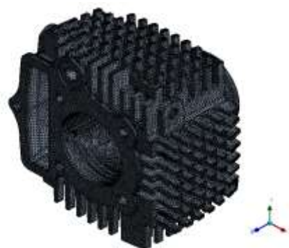
Fig. 11: Meshing of proposed design-1 of engine cylinder block The total node is generated with 803957 and the total number of elements is 455264.
