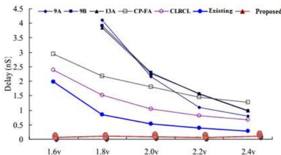
Figure 8: Proposed design performances versus supply voltages (a) Delay.
