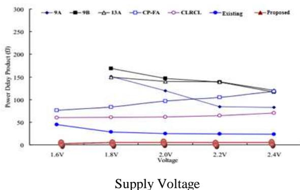
Figure 8: Proposed design performances versus supply voltages (a) Delay. (b) Power-Delay- Product
