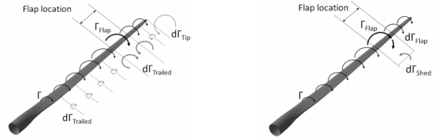
Figure 1: Sketch of bound circulation with trailing and shed vorticity
