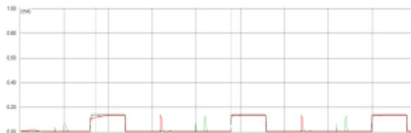
Figure 36: Voltage vs. current simulation in 2 -to-1 MUX with CMOS technique
