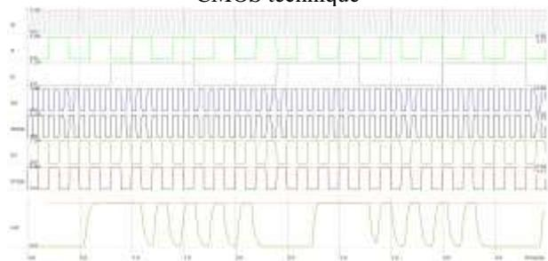
Figure 38 : Voltage vs. time simulation of 4 -to-1 MUX with CMOS technique
