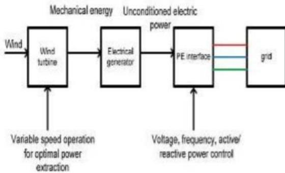
**Figure 1: Variable speed wind energy conversion system**
