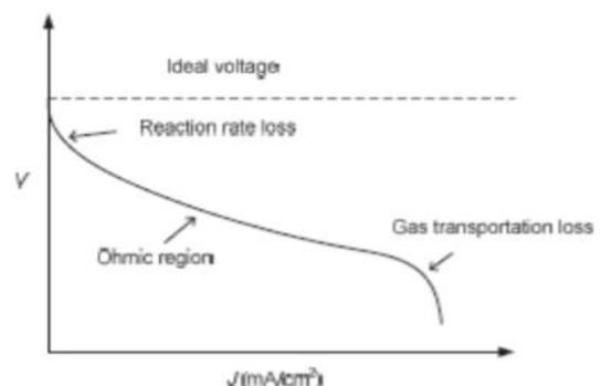
**Figure 3: Typical terminal voltage and current characteristics of a fuel cell [11].**
