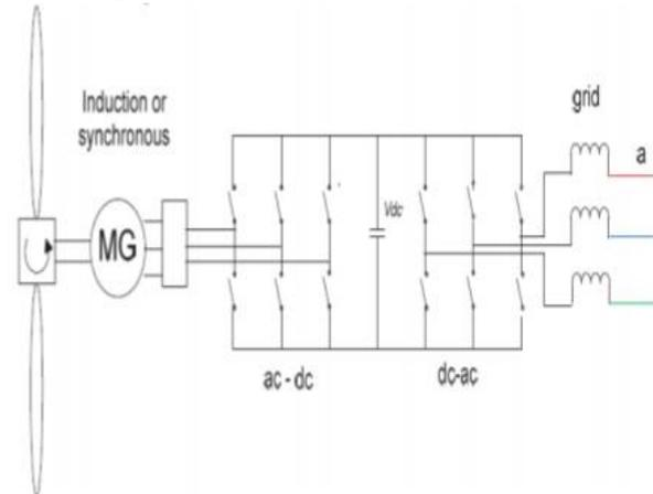
**Figure 2: Fully variable wind energy conversion system**
