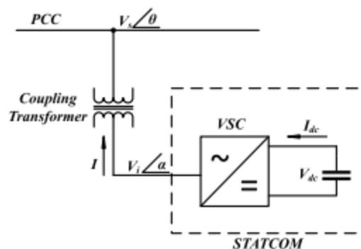
Fig. 3. Schematic diagram of a STATCOM
