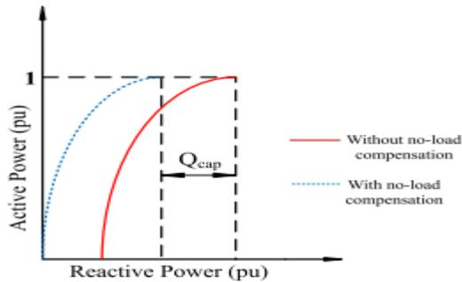
Fig. 2. FSWG reactive power characteristics.
