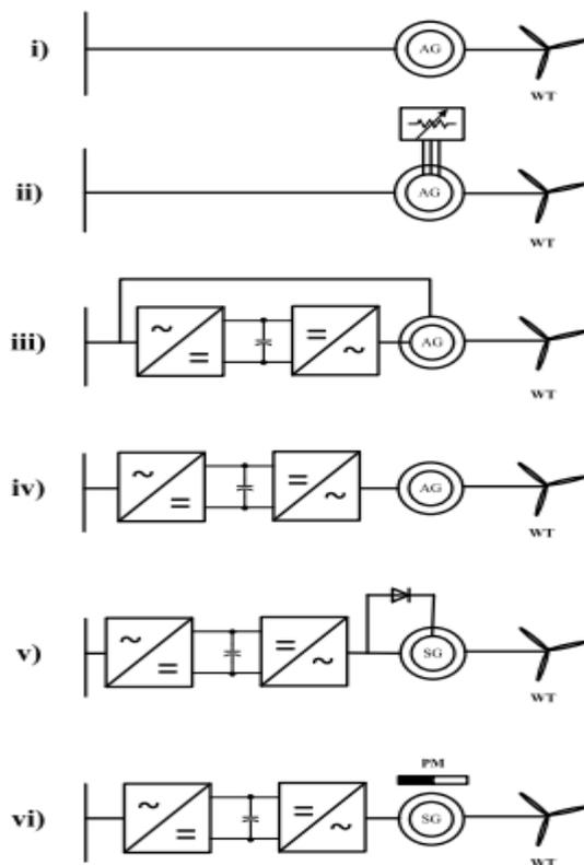
Fig. 1. Typical wind generator configurations: i) Fixed-speed wind generator (FSWG); ii) Limited variable-speed wind generator; iii) Doubly-fed induction generator (DFIG); iv) PEC interfaced fully-fed AG based FCWG; v) Electrically excited synchronous generator based FCWG; and vi) Permanent magnet synchronous generator (PMSG) based FCWG
