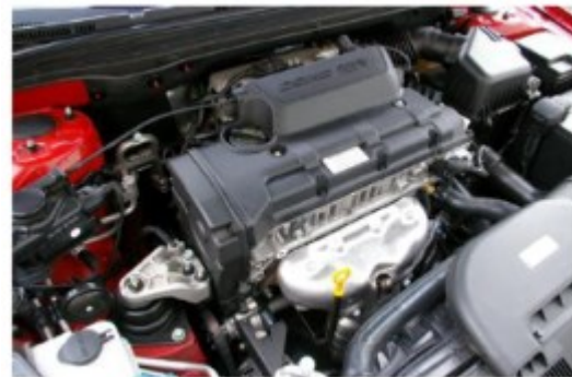
Figure 2: location of engine mounting bracket
