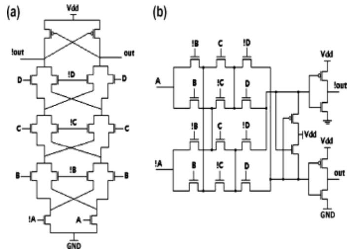
**Fig. 5.** Inverter Design using XOR4 (a) DCVSL and (b) DPTL
