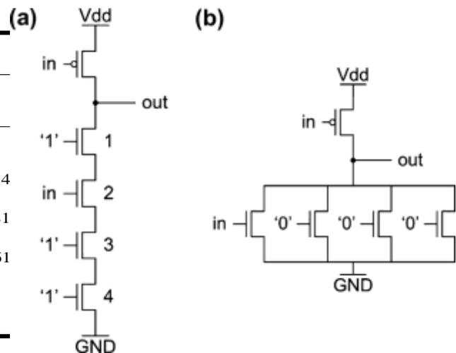
**Figure 4.** Test structures: (a) stacked and (b) parallel devices
