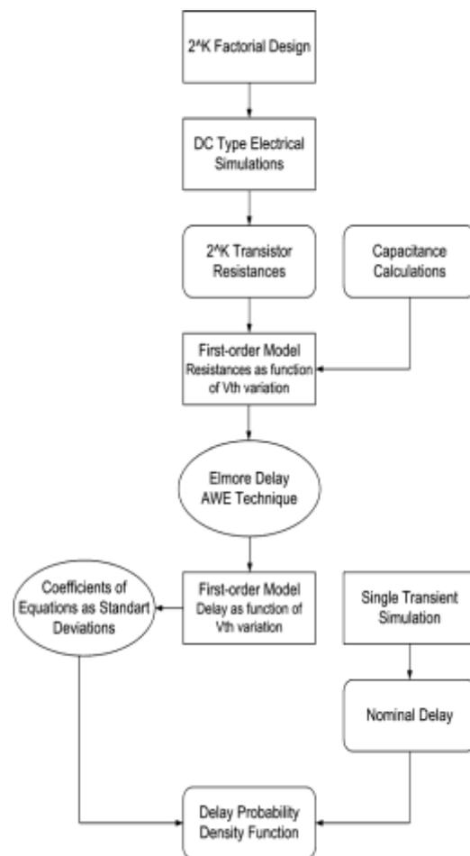
Figure 3 Gate delay variability estimation method flow
