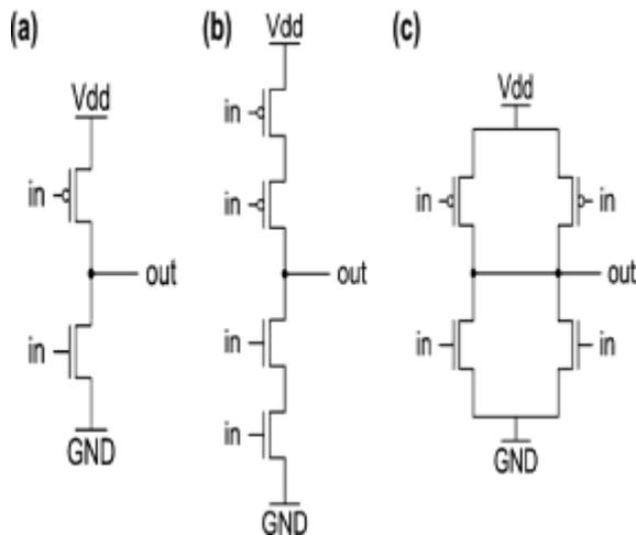
**Figure 5.** CMOS inverters: (a) conventional; (b) low leakage approach; (c) folded topology.
