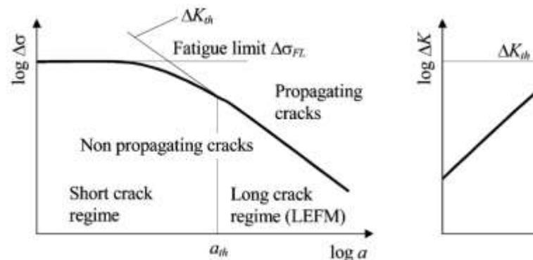
Figure 4: (a) Variation of the applied stress range with the crack length, (b) Variation of the stress intensity range with the crack length
