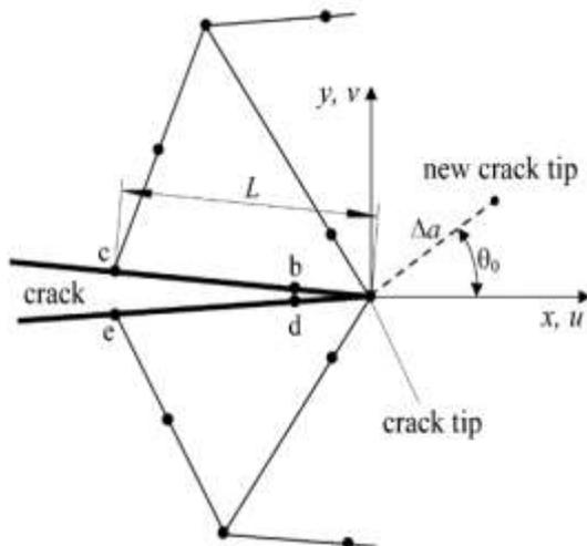
Figure 7: Triangular quarter-point elements around crack tip
