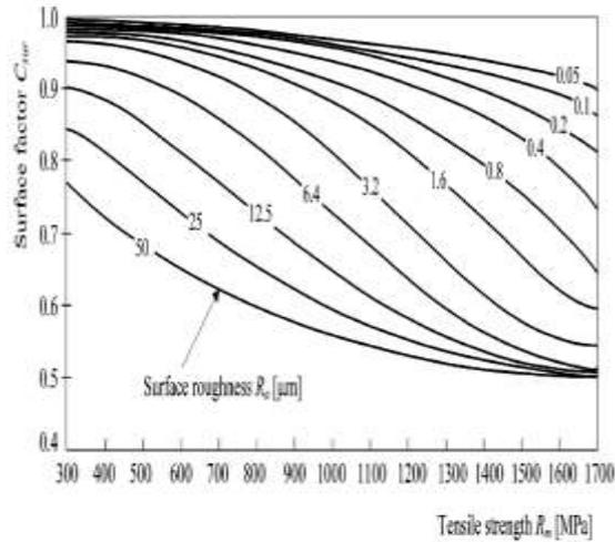
Figure 6: Surface finish correction factor
