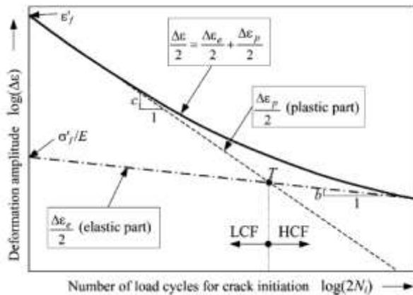
Figure 5: Strain-life ( $\epsilon$ - $N_i$ ) method for the fatigue crack initiation
