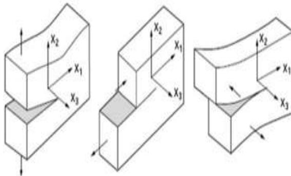
Figure 1: Three types of loading on a cracked body
