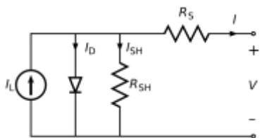
**Fig.1.** Single-diode electrical equivalent of a mono or polycrystalline PV cell
