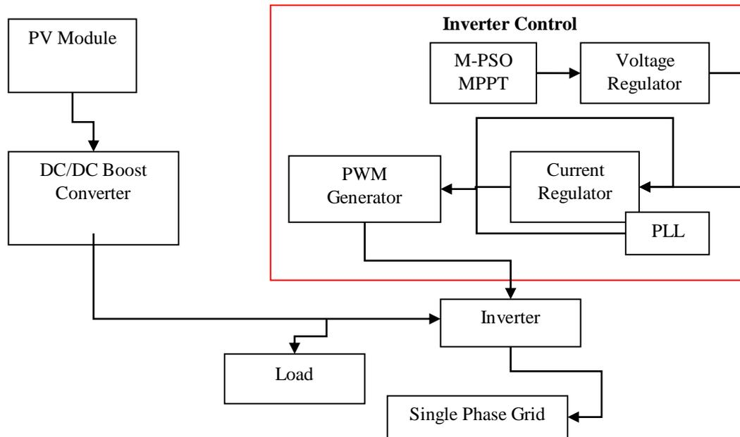
**Fig.4.** M-PSO based Single Phase PV Grid System
