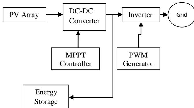
**Fig.3.** Block Diagram of a Solar Power Generation System
