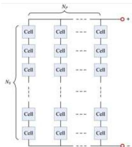
**Fig.2.** Electrical Connection Diagram of a PV Array
