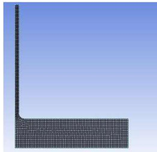
**Fig.3: Meshing: Total No. of Nodes: 1735 & Total No. elements: 1531**
