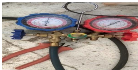
Figure 3 Setup of pressure gauges connected to AC system
