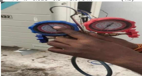
Figure 2 Refrigeration manifold gauge measuring suction and discharge pressure
