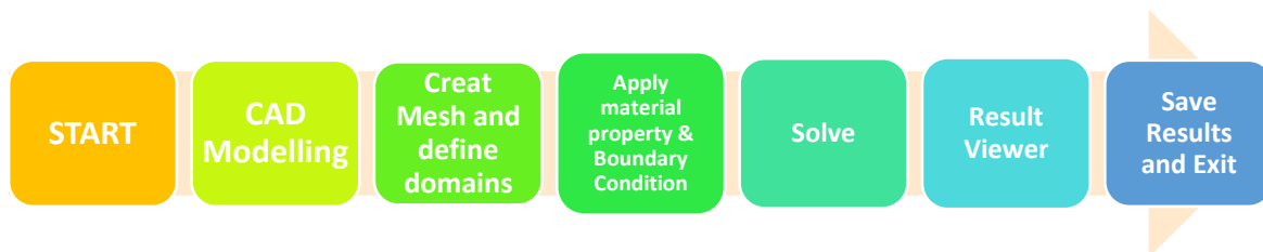
Figure 7 The algorithm utilised for structural and fatigue finite element analysis
