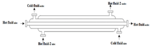
Figure 2 triple concentric-tube heat exchanger [6]
