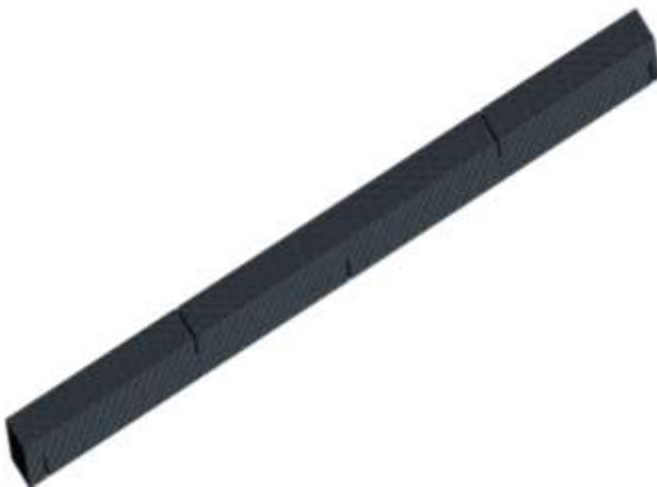
Figure21: Meshing of rectangular shapedamong opposite baffle spacing 120 milimetre& height 15 milimetre Mesh quality: The mesh quality has a significant impact on the calculation's accuracy and stability. Quadrilateral elements were created during discretization in the current study. The accuracy of the answer is influenced by the
