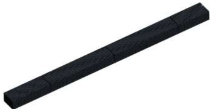
Figure13: Meshing of rectangular shaped with opposite stump spacing 80 milimetre & height 12.5 milimetre As indicated in Figure 13, the overall number of nodes in this work is 378216, and the total number of elements is 346640. Hexahedral elements, which are square in shape and have 20 nodes on each side, are used.
