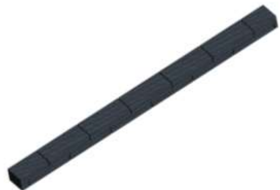
Figure5: Cylindrical channels linking up with opposite flap separation of 40 millimetre and a height of 10 millimetre
