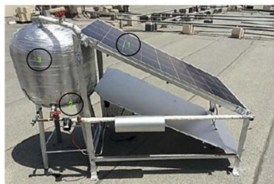
Fig. 3. Hybrid solar Photovoltaic/Thermal (PV/T) cooled by forced water circulation [8]
