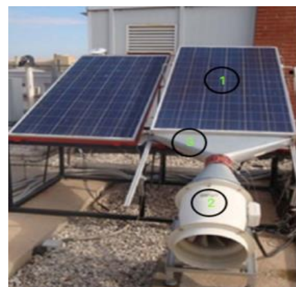
Fig. 6. Hybrid solar Photovoltaic/Thermal system cooled by forced air circulation
