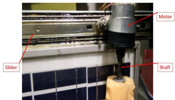
Fig. 10 Setup showing slider, shaft and motor
