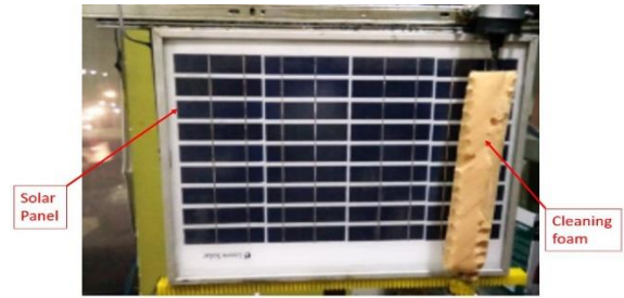
Fig. 9 Setup showing solar panel and cleaning foam
