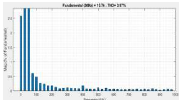
Fig. 17 THD % (0.97%) in current output waveform
