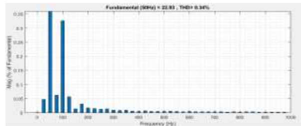
Fig. 27 THD % (0.34%) in current output waveform
