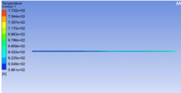
Fig. 8 Temperature contours pipe along longitudinal for case-1
