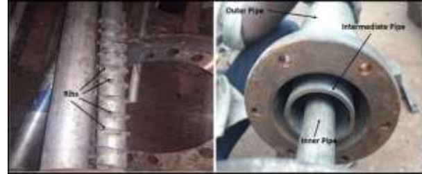
Fig. 1: Arrangement of baffles over the pipe.
