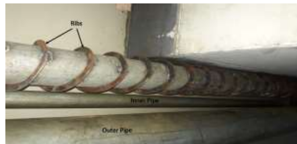
Fig.2: Arrangement of ribs over the pipe.
