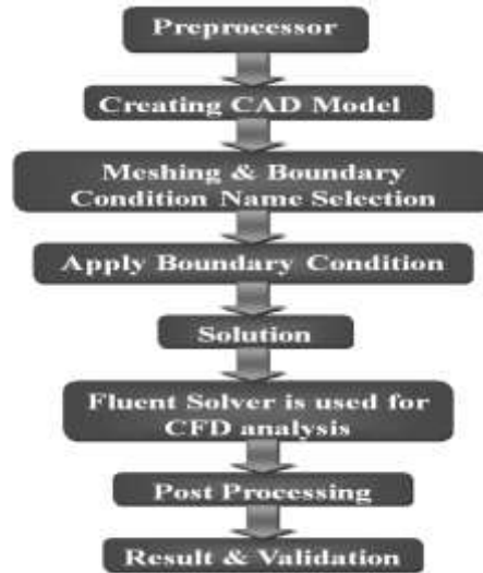
Figure 3: Algorithm used for Computational fluid dynamics analysis
