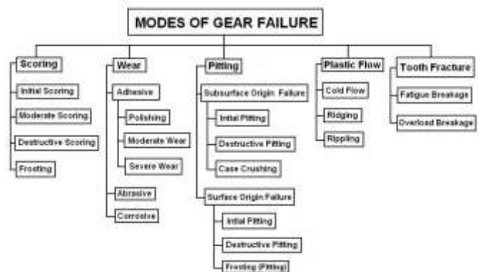
Figure 11: Different modes of failure
