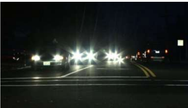
Figure 2: Glaring Effect due to Upper Mode of Headlight
