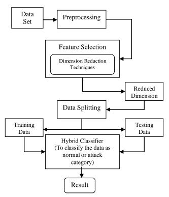
Figure 1: Proposed Flow Diagram of Intrusion Detection System
