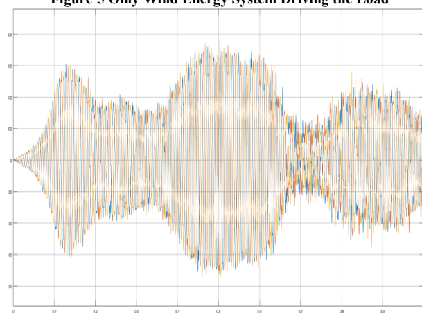
Figure 6 Voltage output from wind energy system only with 500KW load
