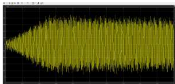
Figure 27: Active Power Output from the inverter with Vector Modulation
