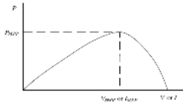
Figure 5: Characteristic PV array power curve
